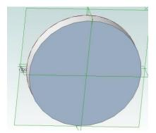
Radius of disk = 3.937", thickness=1" Internal heat generation =  $10 \text{ BTU/(s.in}^3)$ k = 0.01375(1 + 0.001T) = 0.0203 BTU/(s.in.F)
