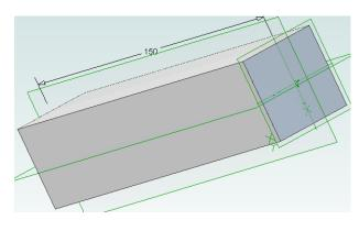
Length = 150mm Width = 30mm = Thickness Thermal conductivity, k = 0.9e-3
