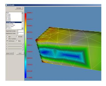
• As we inspect the new solution, we notice that the stresses at this end are exactly what we would expect from theory – there is a clear area of near-zero stress in the center of the beam (the "neutral axis"), and the stress is highest at the corners of the cantilever end, i.e. the points with the highest bending moment that are also farthest away from this neutral axis
