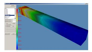
Instead of sharp lines between the color bands representing different stress values, we can smooth out these colors with the "Continuous" check box
